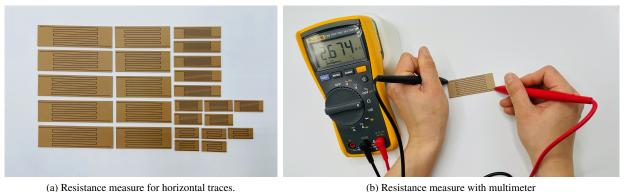
Figure B.2: Serpentine trace patterns printed to measure the horizontal traces' resistance.
